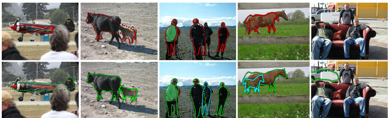
Fig. 8 Comparison results of object detection on a subset of PASCAL dataset. The top / bottom row showing the results by the method without / with part importance (Color figure online)
