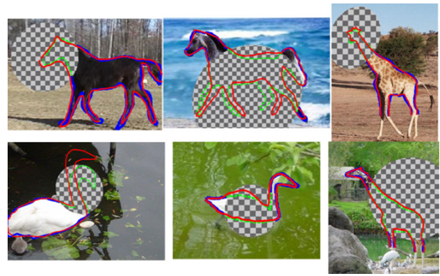
Fig. 4 Shape completion examples. The blue contour segments are the object boundaries not been occluded. The red shapes denote the reconstructed contours by the proposed shape reconstruction method. The dotted green curves are the occluded ground truth object outlines. The regions of chessboard pattern are the occlusion masks (Color figure online)
